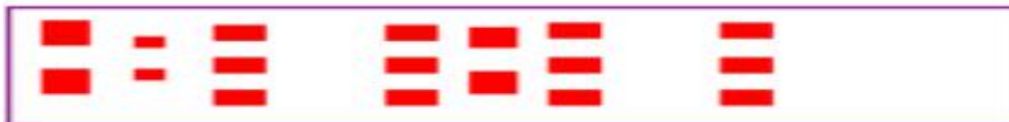
顶层阻焊 TOP SOLDER
